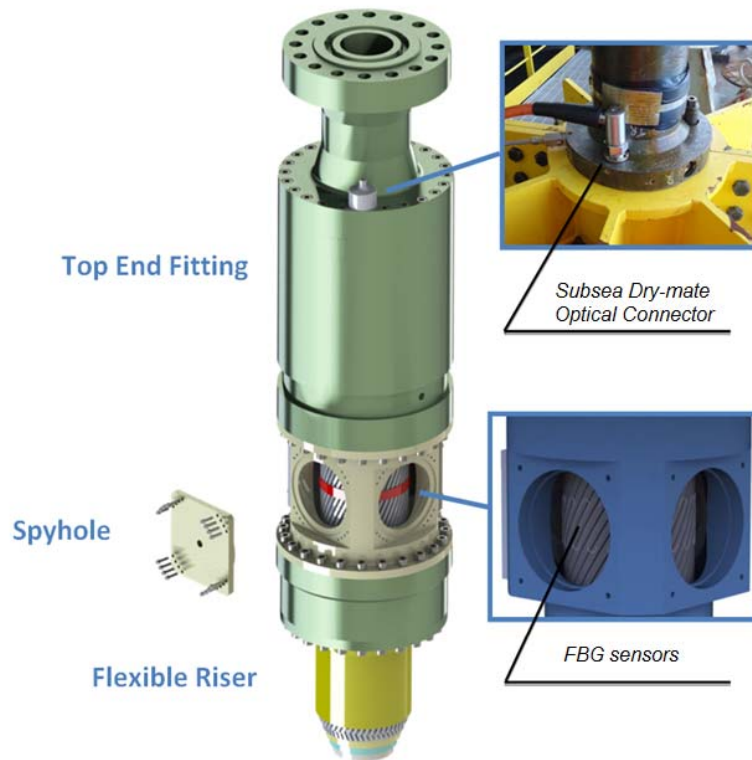
Figure 2 – Spyhole End Fitting with MODA sensors.
