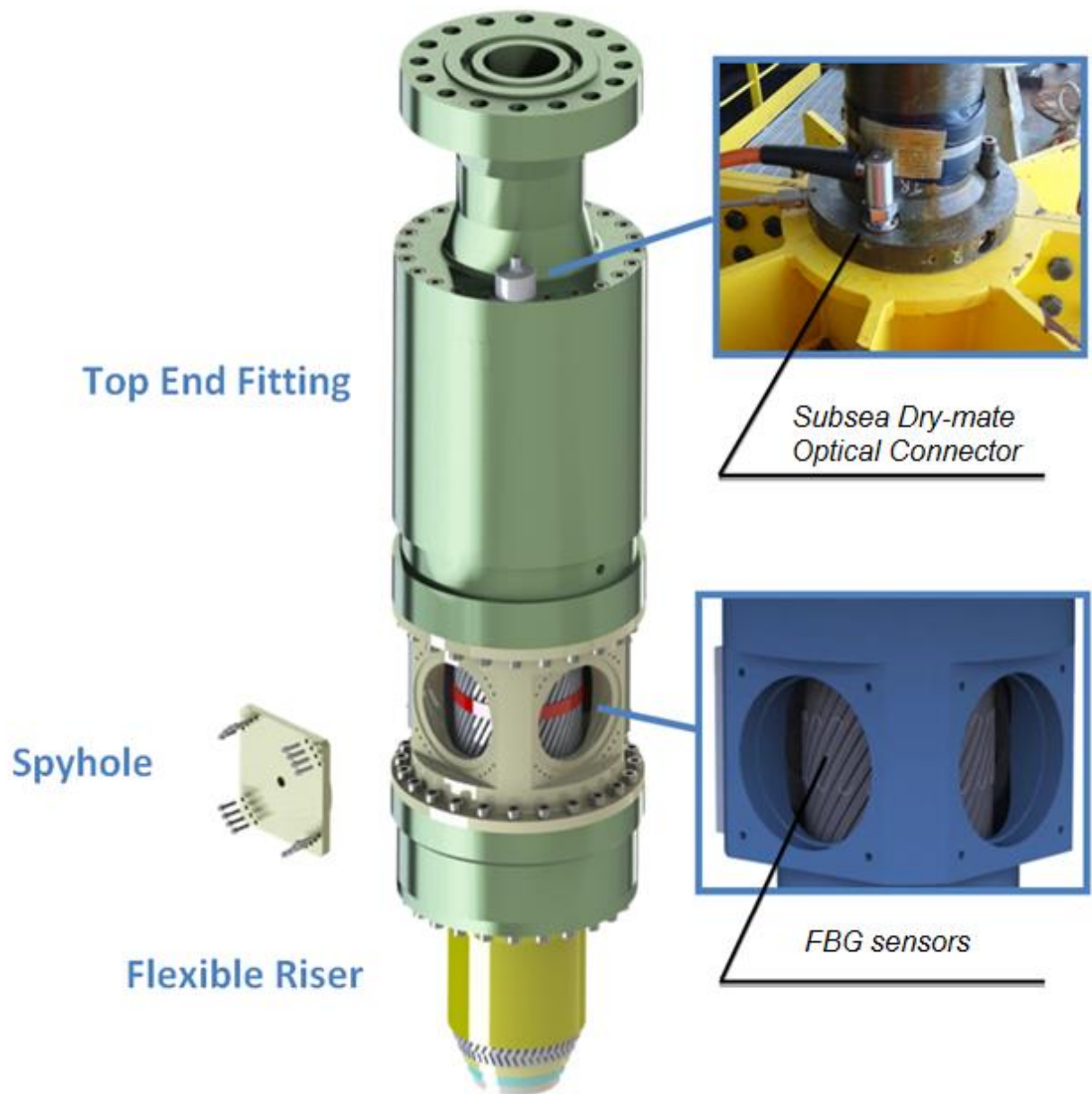
Figure 1 – Spyhole End Fitting with MODA sensors.
