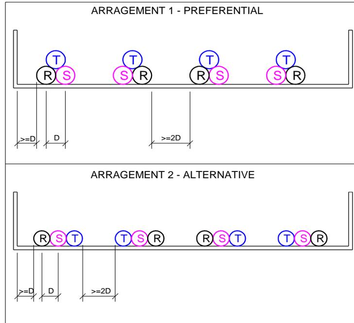
Figure 4 - Single-Core Cables Arrangement
