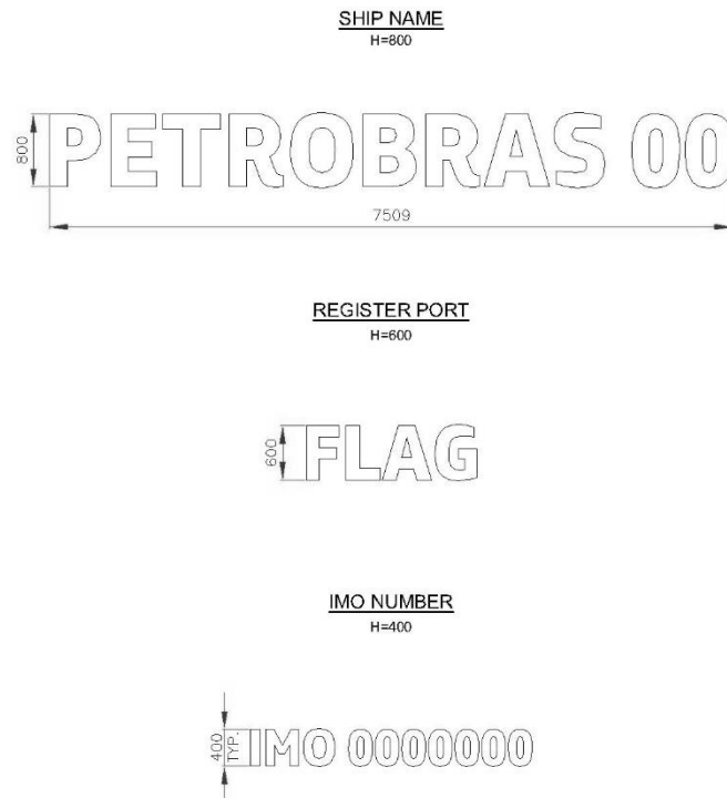
Figure 3 - Detail of letter type of transom marks (FPSO name, port of registry and IMO number)
