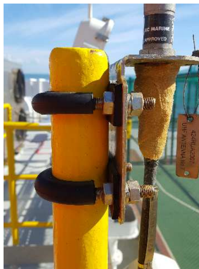
Figure 2: Insulation to avoid galvanic corrosion.
