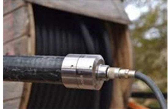
Figure 13: Connection between RF cable and RF flexible tail
